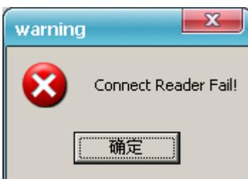
If the T-75 can't connect to PC through the USB, or the selected serial port is wrong, the connection will fail.
