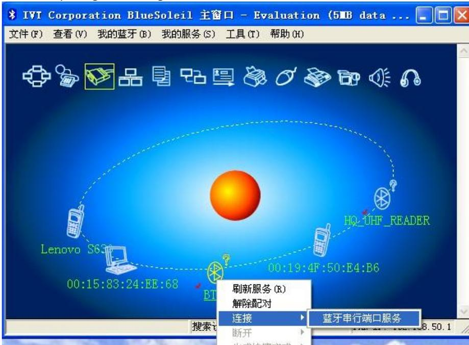
At this time, the Bluetooth management tools will automatically connect with T-75 by Bluetooth adapter. The same time, the specific serial port service information in the system file shows the COM port number. As below:
