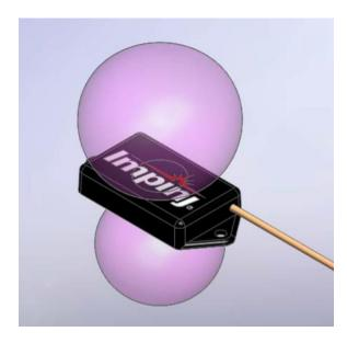
The MatchBox antenna emits RF energy from both the top and bottom surfaces. Tags are essentially unreadable beyond 5 cm from the antenna surface
